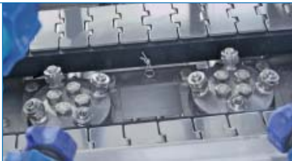
Top: Arrangement of spraying nozzles and external detergent tank
