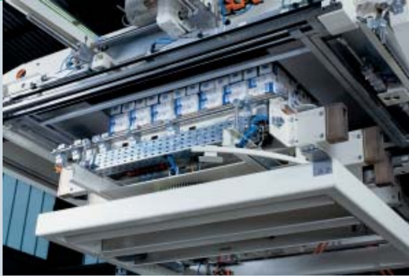
The Innopal PBHS palletizing complex layer patterns
