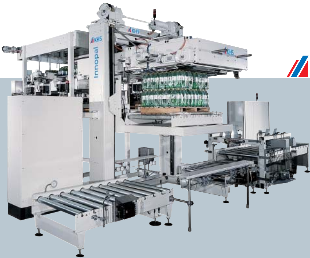
Pallet lift to the top loading position
