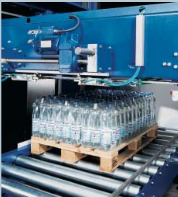
Motor-driven layer centering
