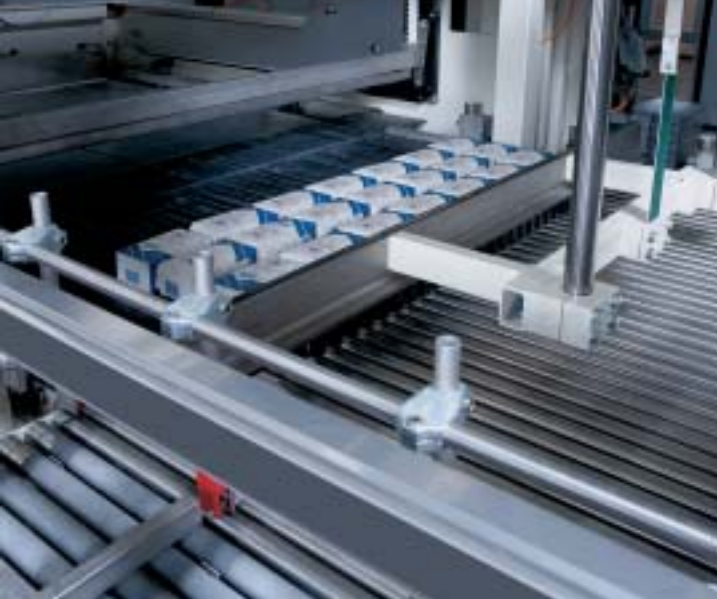
Grouping station row pusher
