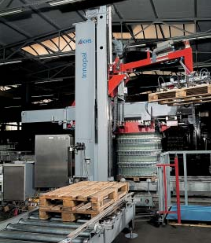
Innopal ASN with handling robot for pallet manipulation
