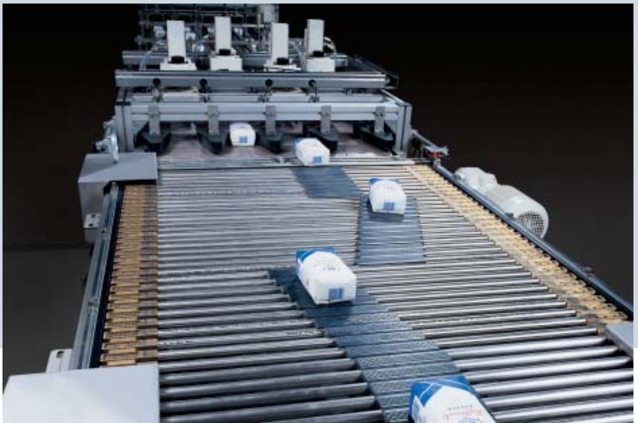
Infeed to the turning facilities
