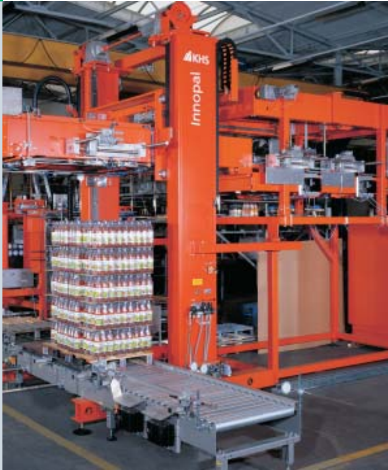
Innapal PBN palletizing robot with grouping station
