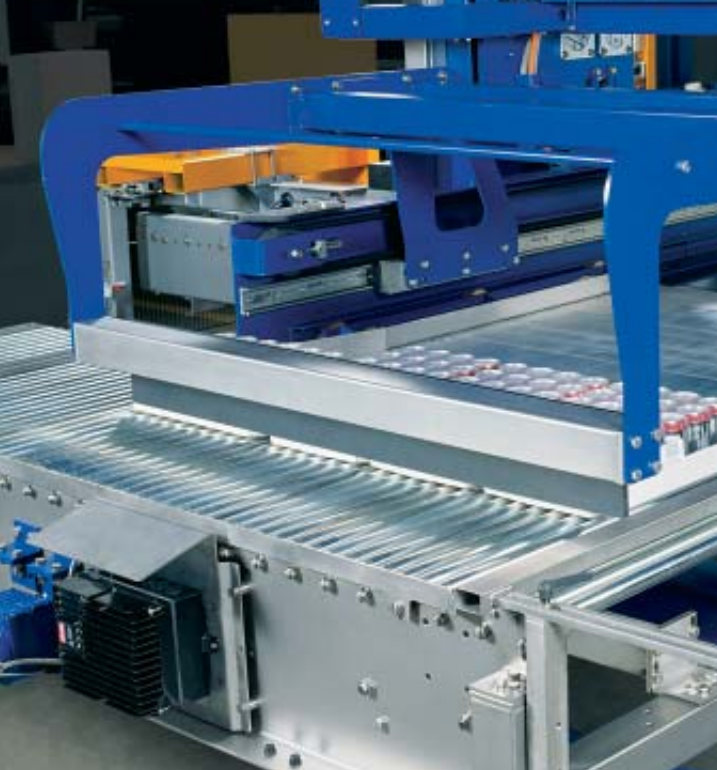
Frequency controlled infeed roller conveyor
