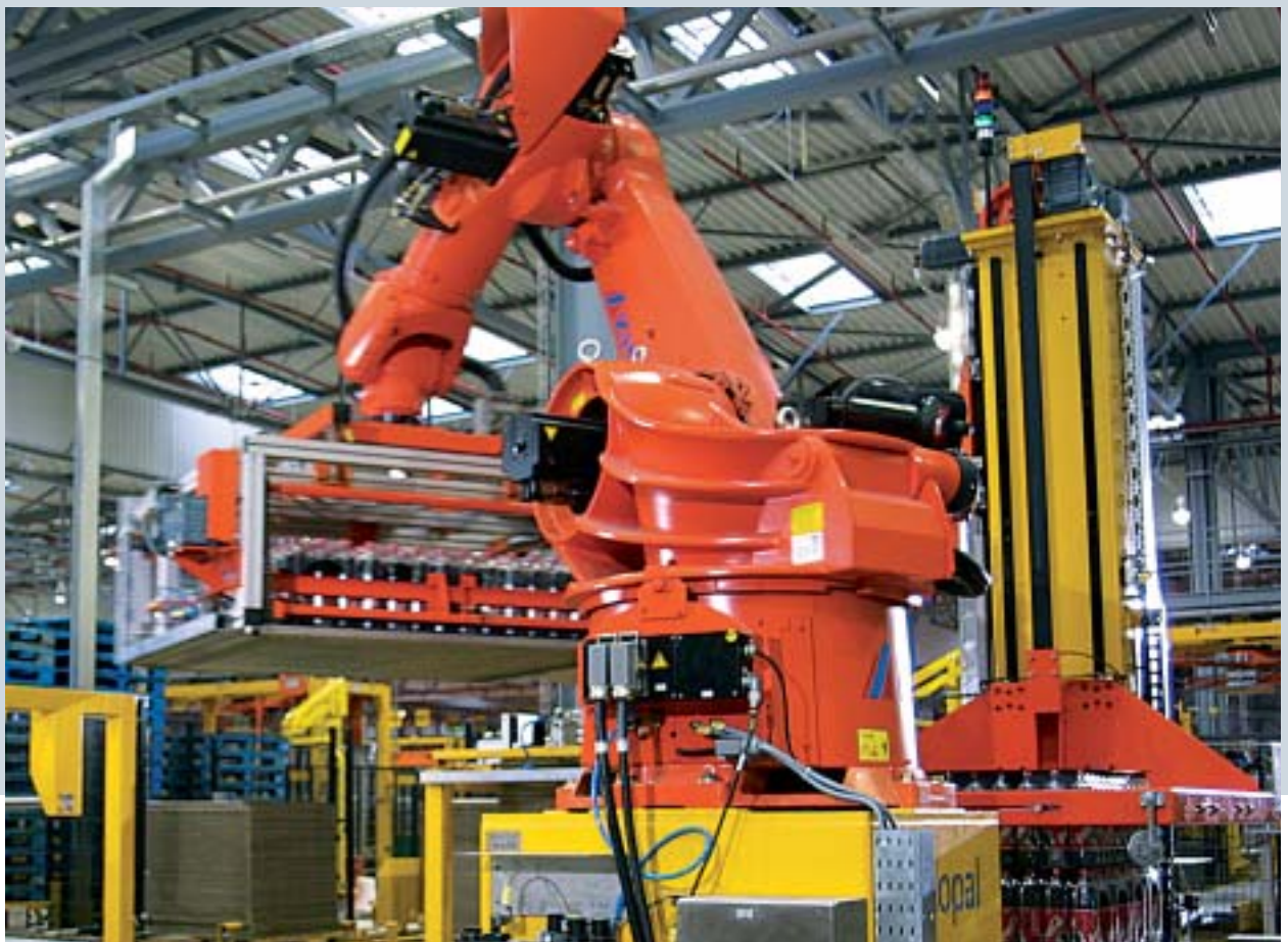
Innopal RK with roller carpet and Innopal RSZ column-type centering
