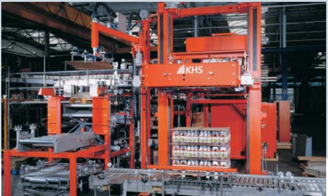
Innapal PBN 1 processing half pallets with a handling robot for inserted liners
