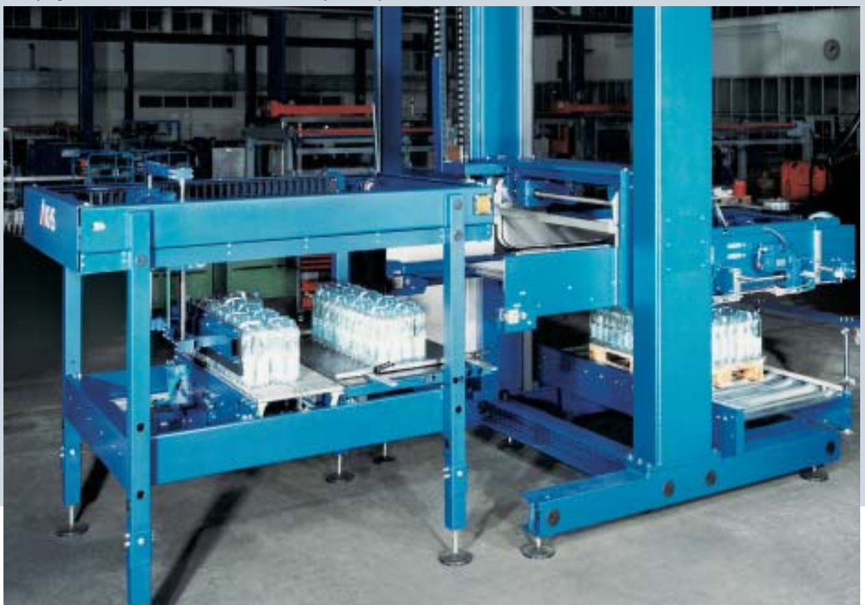
Grouping station with low-level infeed to an Innapal PBN palletizer
