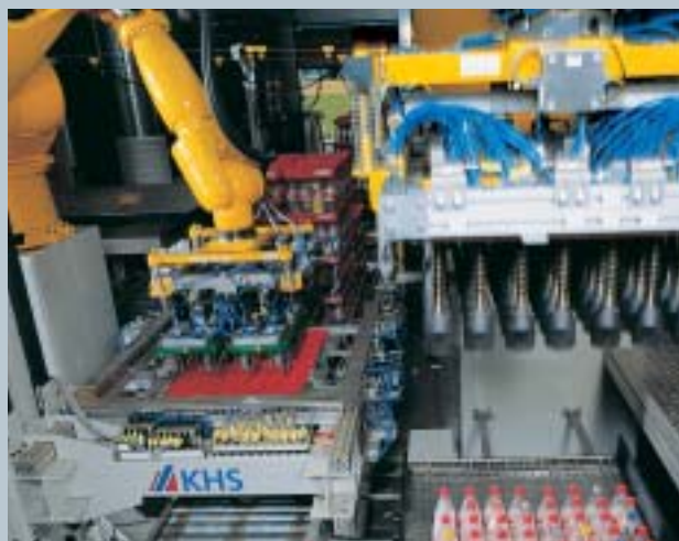
Highly flexible combined packer/palletizer for processing displays
