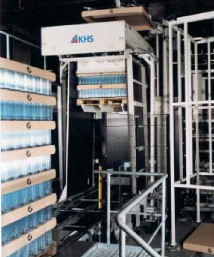
Pallet lift with partially depalletized new glass pallet
