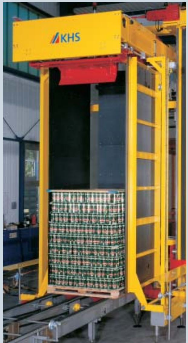
Lift well with three-sided centering
