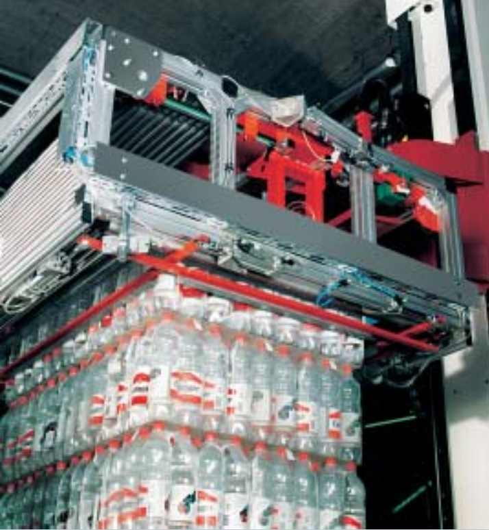
Four-sided centering of the last layer while pulling out the roller carpet
