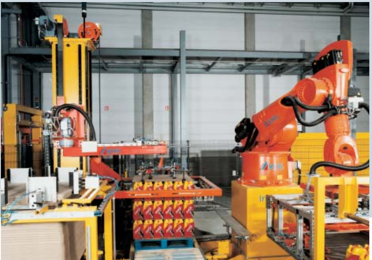
Innopal RSZ together with an Innopal RK palletizing robot
