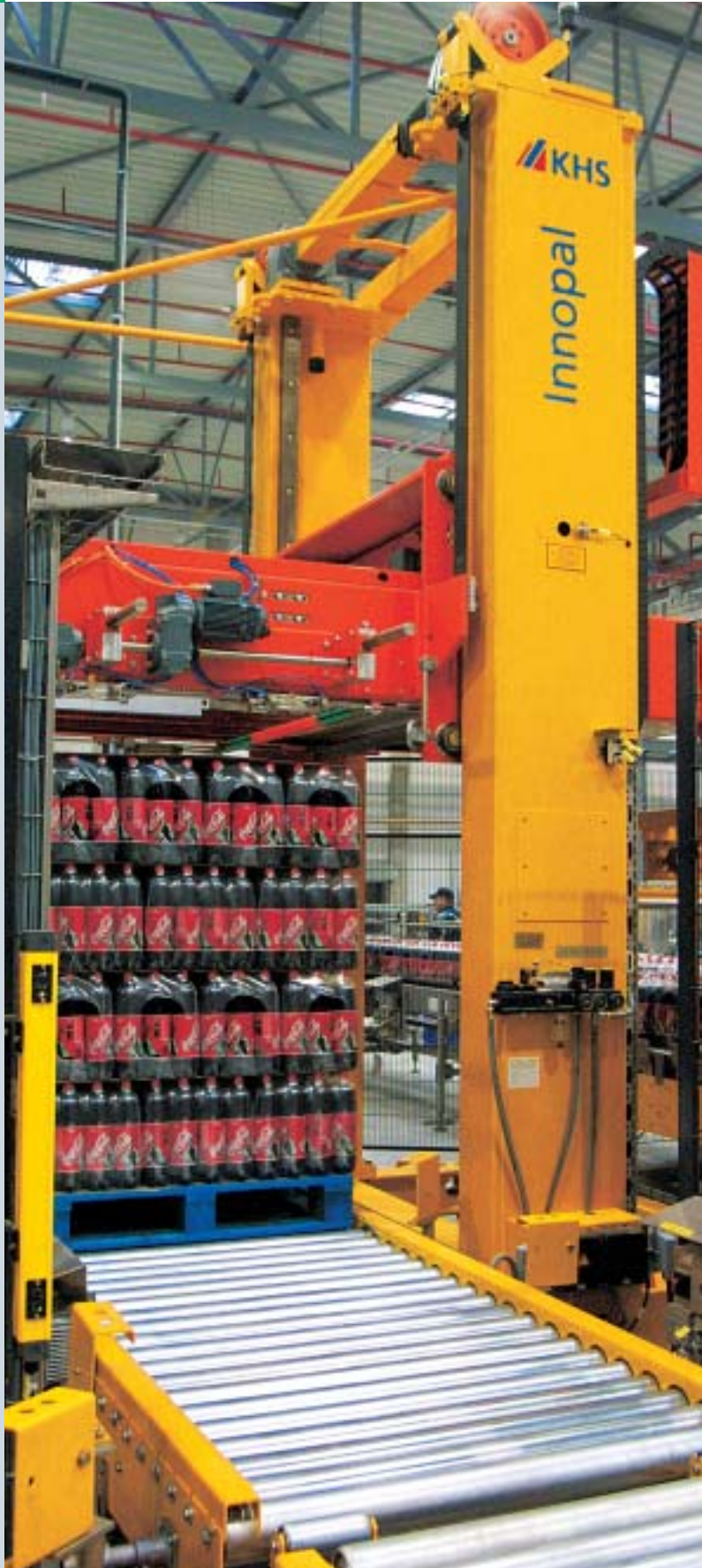
Palletizing process at the Innopal PBN 1
