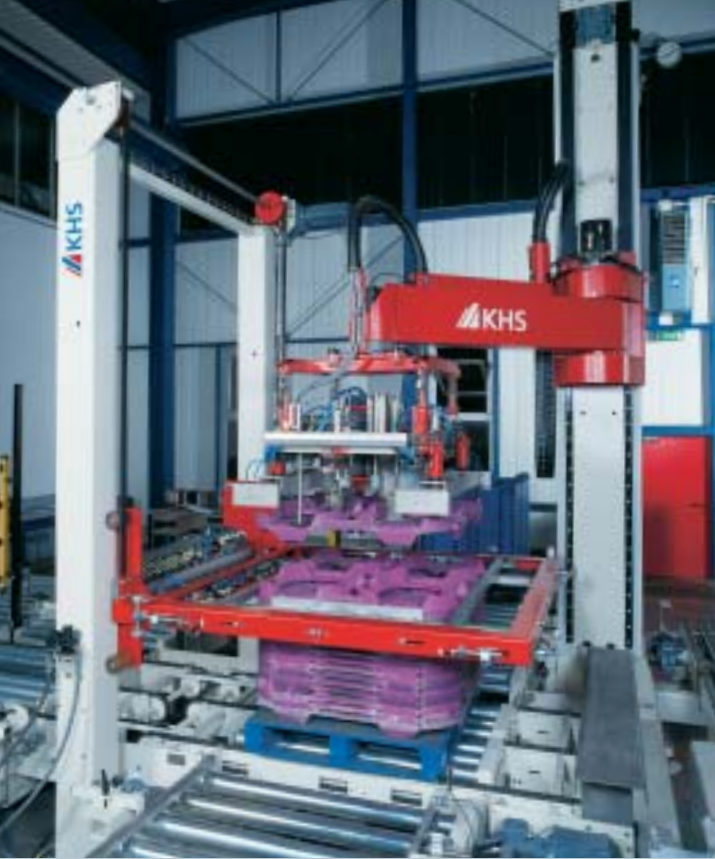
Innopal RS 3 aided by gantry-type centering
