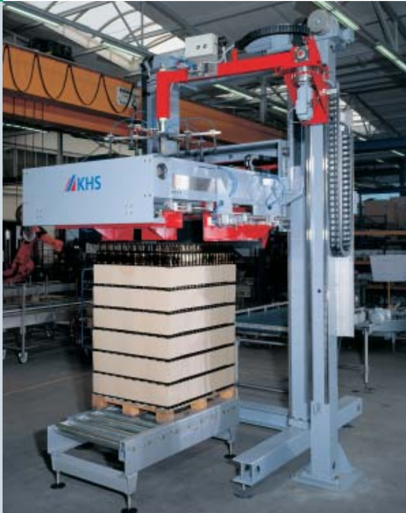
Free-standing handling robot at a depalletizer equipped with height control
