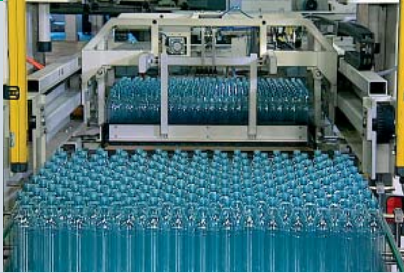
Pushoff and container discharge of an Innapal ASH
