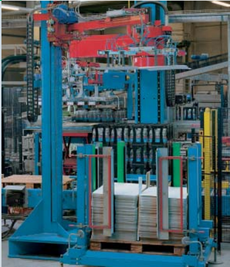
Innapal HR handling robot processing inserted liners for two half pallets each
