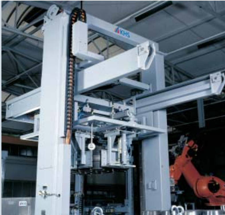
Innapal PKN with fixed cross-conveying
