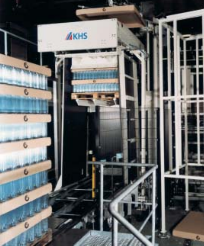
Partially depalletized empties pallet
