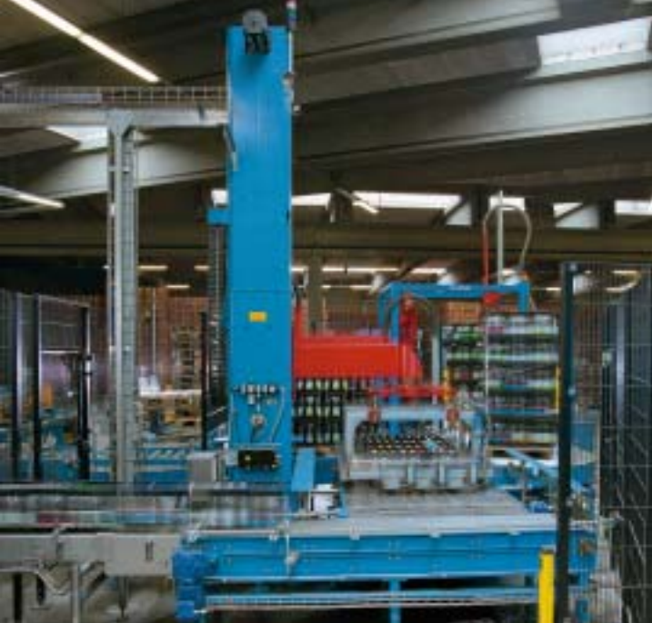
Clamping head of an Innopal RS 3 depalletizer
