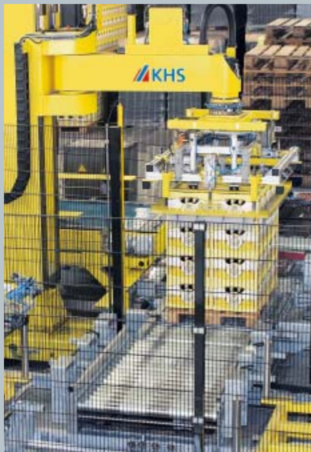
Individual lengthwise and crosswise clamping of each row
