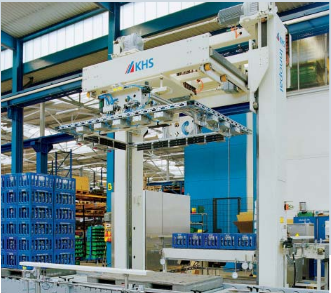
General view of an Innapal PKTN 1 returnables palletizer
