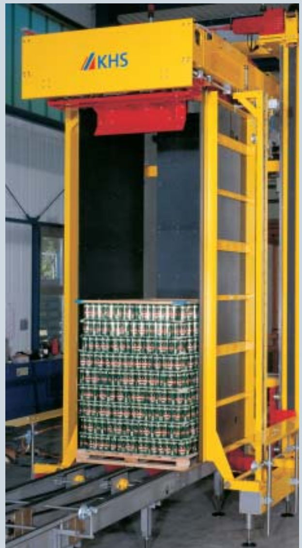
Three-sided guidance of empty container pallets in the lift well of the Innapal ASH
