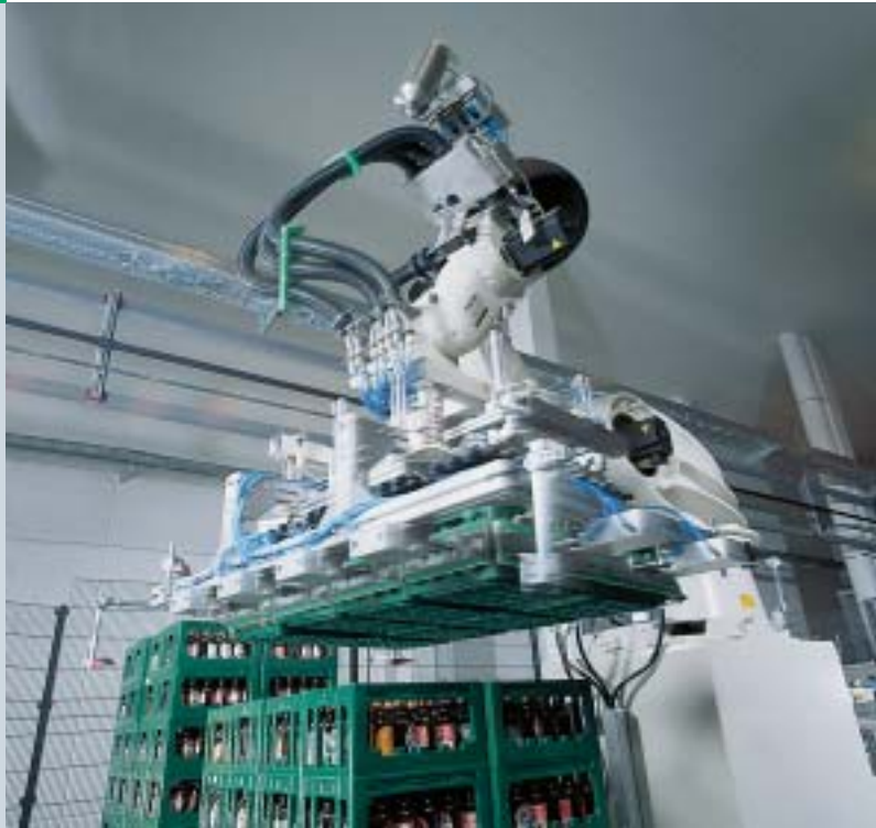
Innapal RK depalletizer and clamping head
