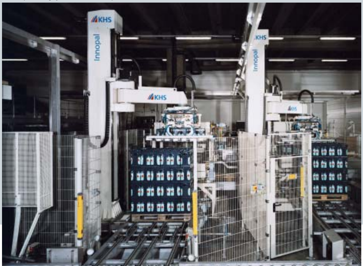
Double palletizing system with two Innopal RS 3 robots
