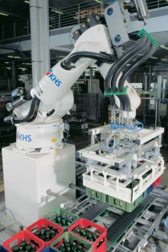
Whole-layer pack discharge of an Innopal RK depalletizer
