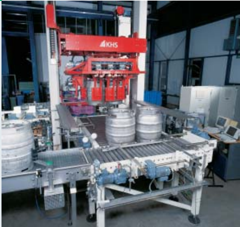
Innopal PKTN 1 with telescopic cross-conveying
