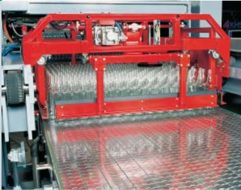
Partially depalletized empties pallet
