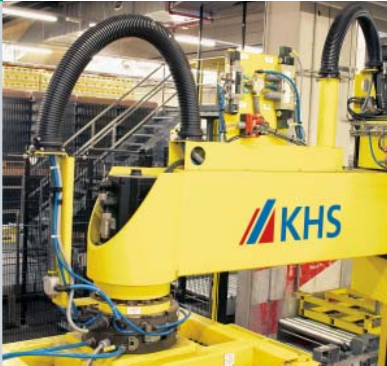
Gripper head with full crates in an Innopal RS 3
