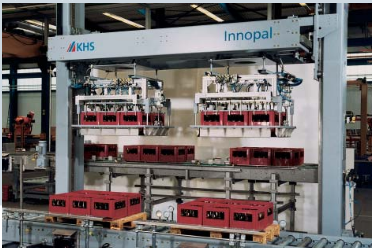
Innopal PKTN 2 with gripper head for full packs
