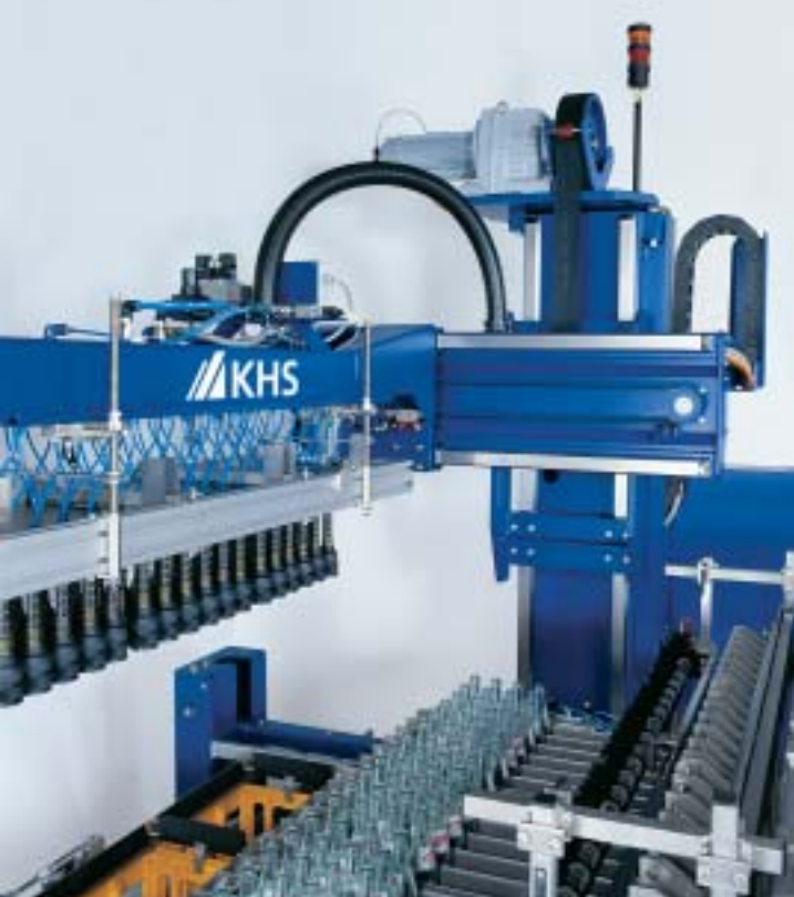
Packing head guidance on linear units without play
