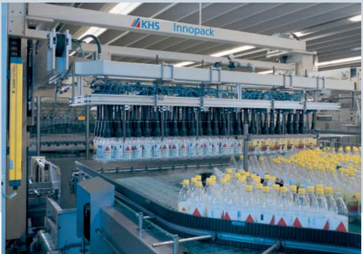
Selective unpacker for mixed no-return and non-refillable deposit PET
