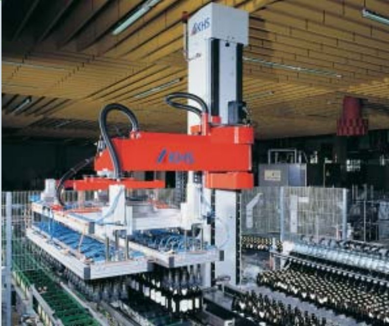
Innopack RS 3 as a combined packer: Packing and unpacking at each cycle
