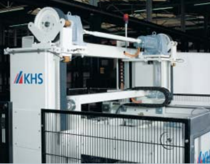
Fast-running shaft between the gears for precision synchronous operation
