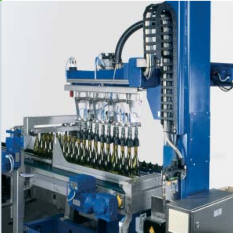
Lifting column, lift unit with infeed table, here: H-shaped layout
