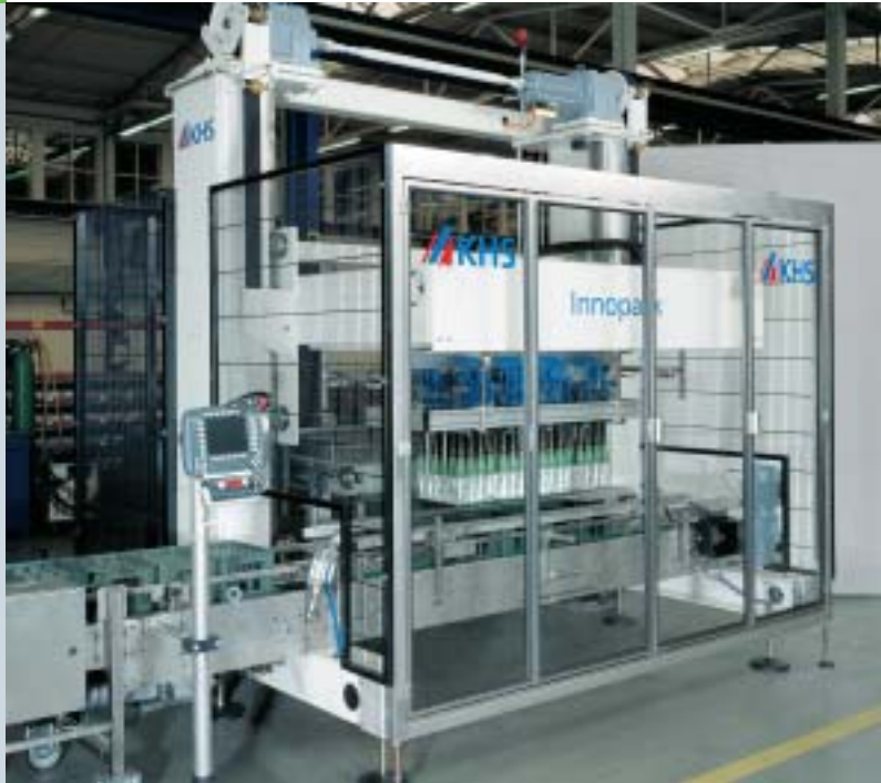
Economical enclosure of the Innopack PPZ; operator panel equipped with visualization and operator prompting
