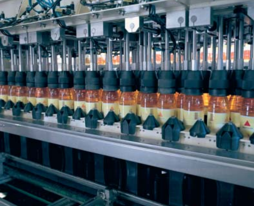
Sensory equipment (bottom) and motors (top) at the alignment head
