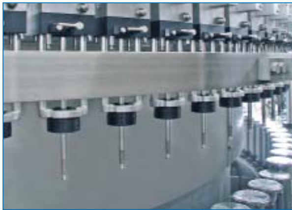
Filling valves with only a few mechanical parts. Little servicing effort. Long service life.
