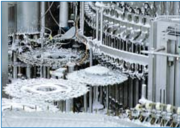
Exterior sanitizing of the filler block. Foam and flushoff cleaning at predefined time intervals. Top-level spotless cleanliness.
