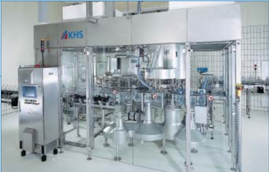
Freestanding machine enclosure Made entirely of glass or Makrolon. Great transparency. Complete runoff of cleaning media. High hygienic safety.
