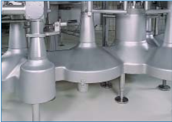
Hygienically designed front table. No niches, dead spaces, corners, edges. High-level ease of external sanitizing.
