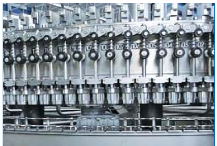
Innofill DMD – fill levels centrally set by adjusting the height of the ring bowl
