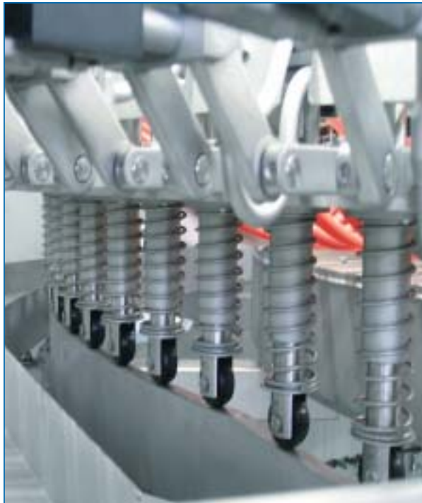
The cam-controlled spray tube
